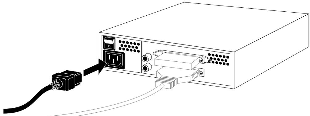
**Figure 5-9** Connecting the Power Cable to an External Device
