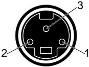
Figure A-14 Stereo View Port Pinout Assignments
