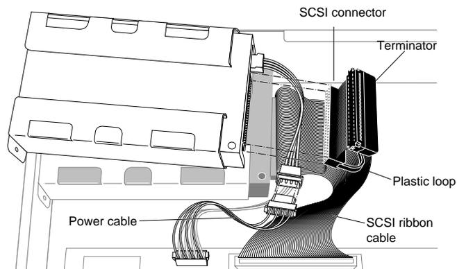
**Figure 8-29** Disconnecting the Power and SCSI Cables From the Floptical Drive
