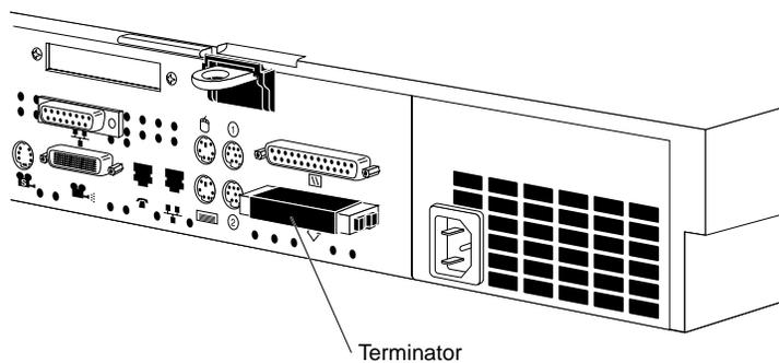
**Figure 5-5** Removing the SCSI Terminator From the Indy Workstation
