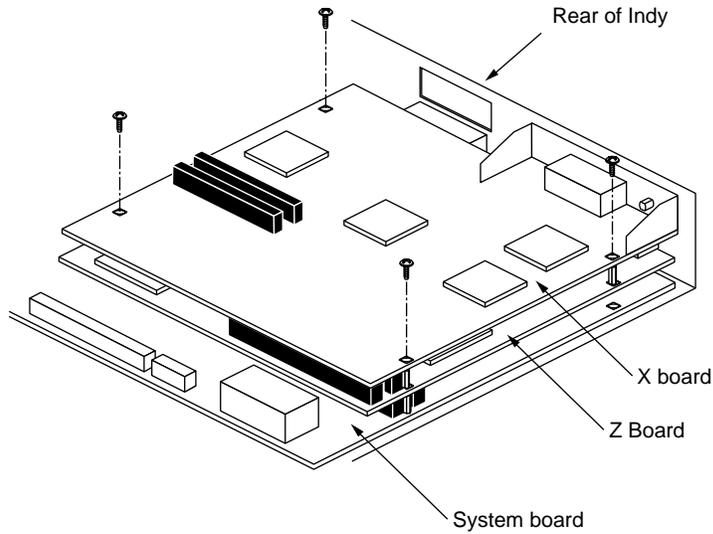
**Figure 8-14** Removing the Screws From the X Board
