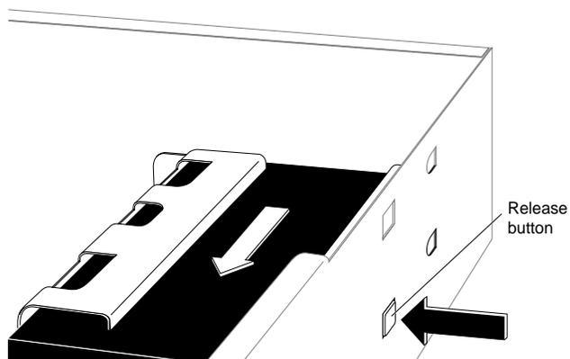
**Figure 8-33** Removing the System Disk Drive
